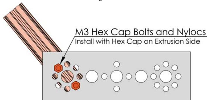
**Figure 60: Mounting 15mm Extrusion to Tetrax Channel**
