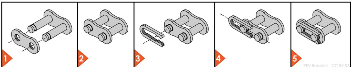
Figure 36: Master Link Detailed Assembly for Reference
