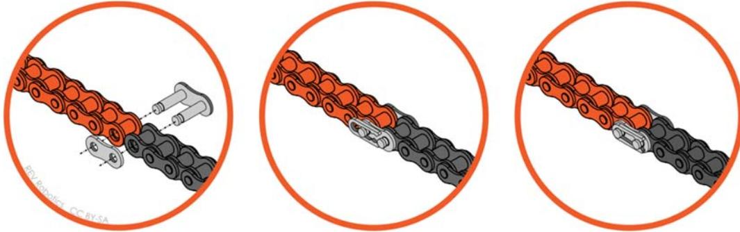
Figure 38: Master Link Assembly on Chain
