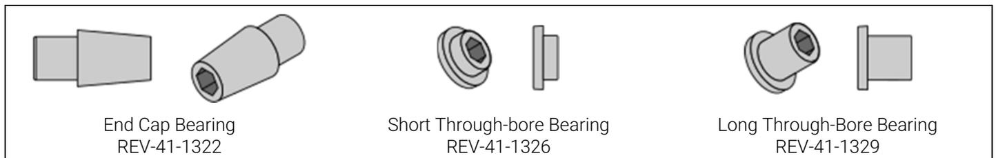
**End cap bearings** are closed on one end, so when these bearings are placed on both ends of a shaft and fit into motion brackets the shaft is free to rotate but is fully constrained laterally (sideways).
