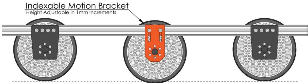
Figure 46: Drop Center Wheel Using an Indexable Bracket
