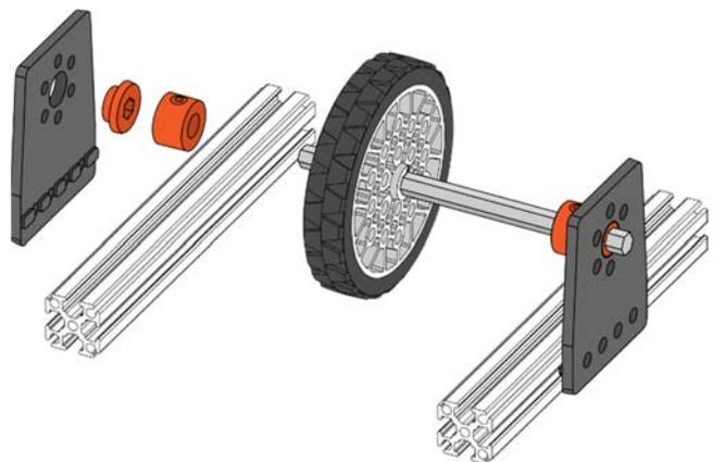
Figure 9: Motion Bracket and Short Through bore Bearings
