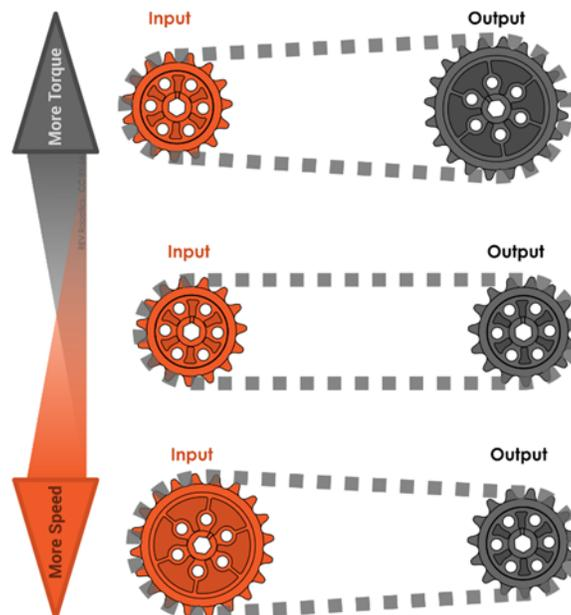
Figure 31: Using Sprockets to Increase Speed or Torque
