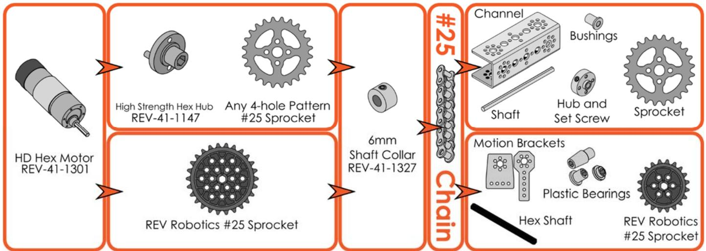
Figure 56: Sprocket and Chain Drive with Hex
