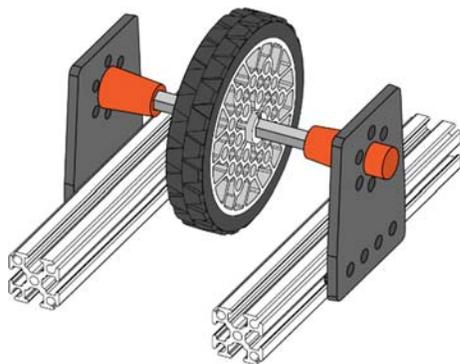
Figure 8: Motion Brackets and End Cap Bearings
