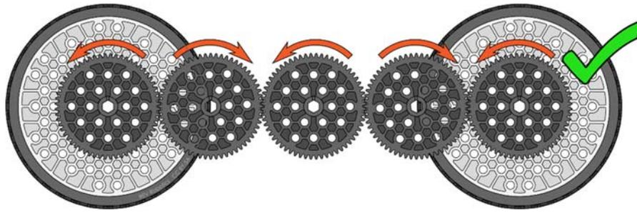
Figure 48: Correct All Gear Drivetrain
