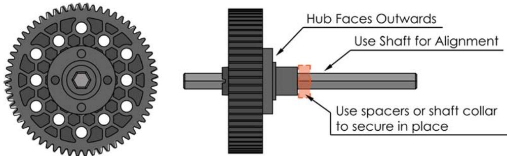
Figure 23: Hex Hub Adapter Mounted on a REV Gear for Added Strength
