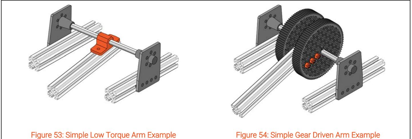
Figure 53: Simple Low Torque Arm Example
