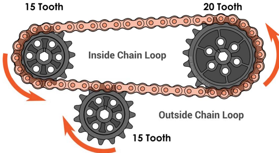
Figure 51: Single Stage Reduction (15:20) with Idler
