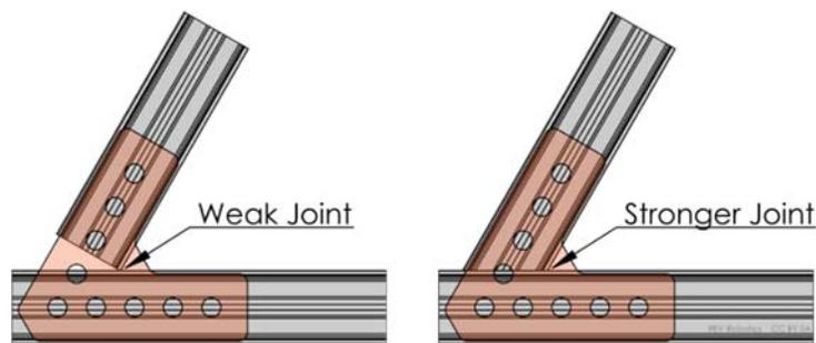
Figure 13: Extrusion with Beveled Joint
