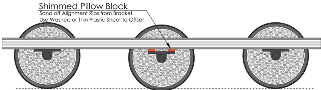
Figure 47: Drop Center Using a Shimmed Pillow Block
