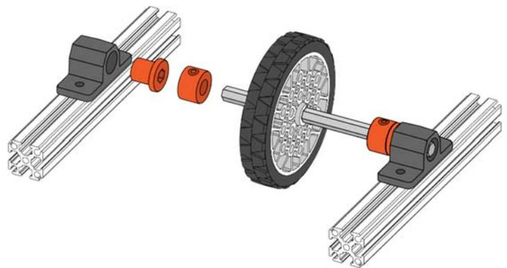
Figure 11: Pillow Blocks and Long Through bore Bearings
