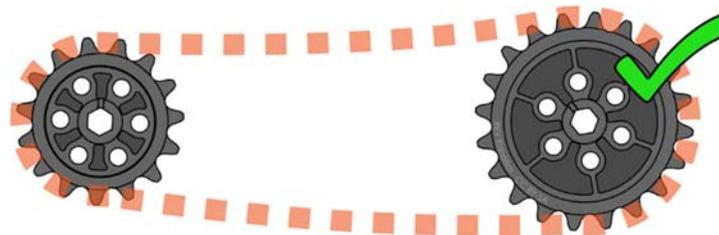
Figure 33: Correctly Spaced Sprockets (Chain Correctly Tensioned)
