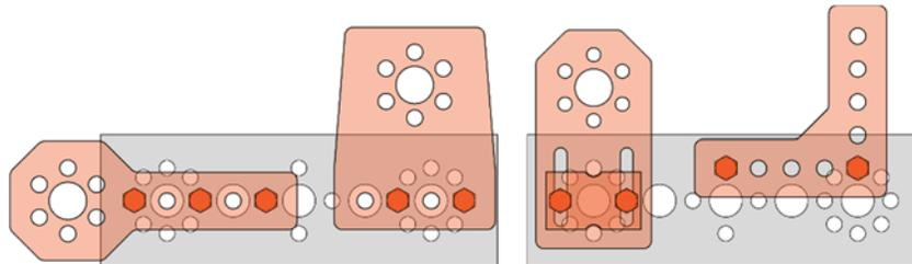
**Figure 59: Mounting REV Robotics Brackets to Tetrax Channel**
