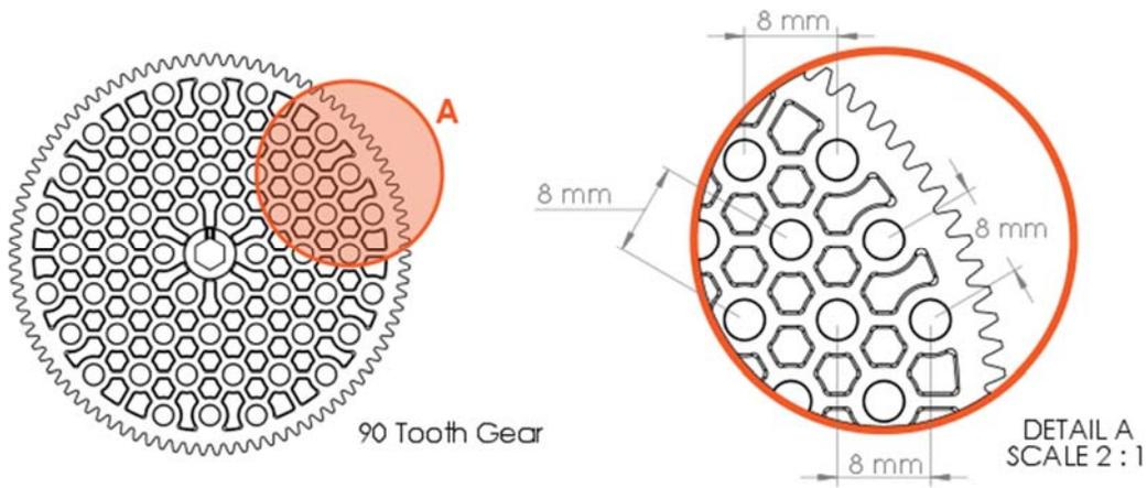
Figure 26: Motion Component Bolt Pattern Detail
