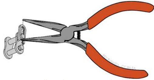
Figure 37: Installing the Master Link Clip with Pliers
