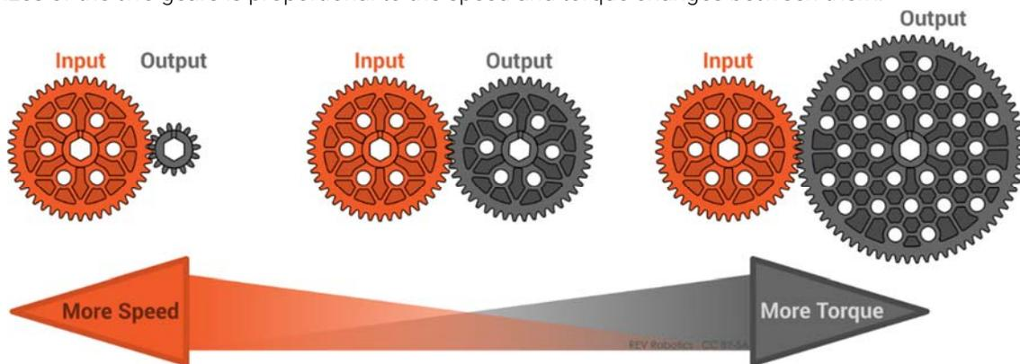
Figure 39: Using Gears to Increase Speed or Torque
